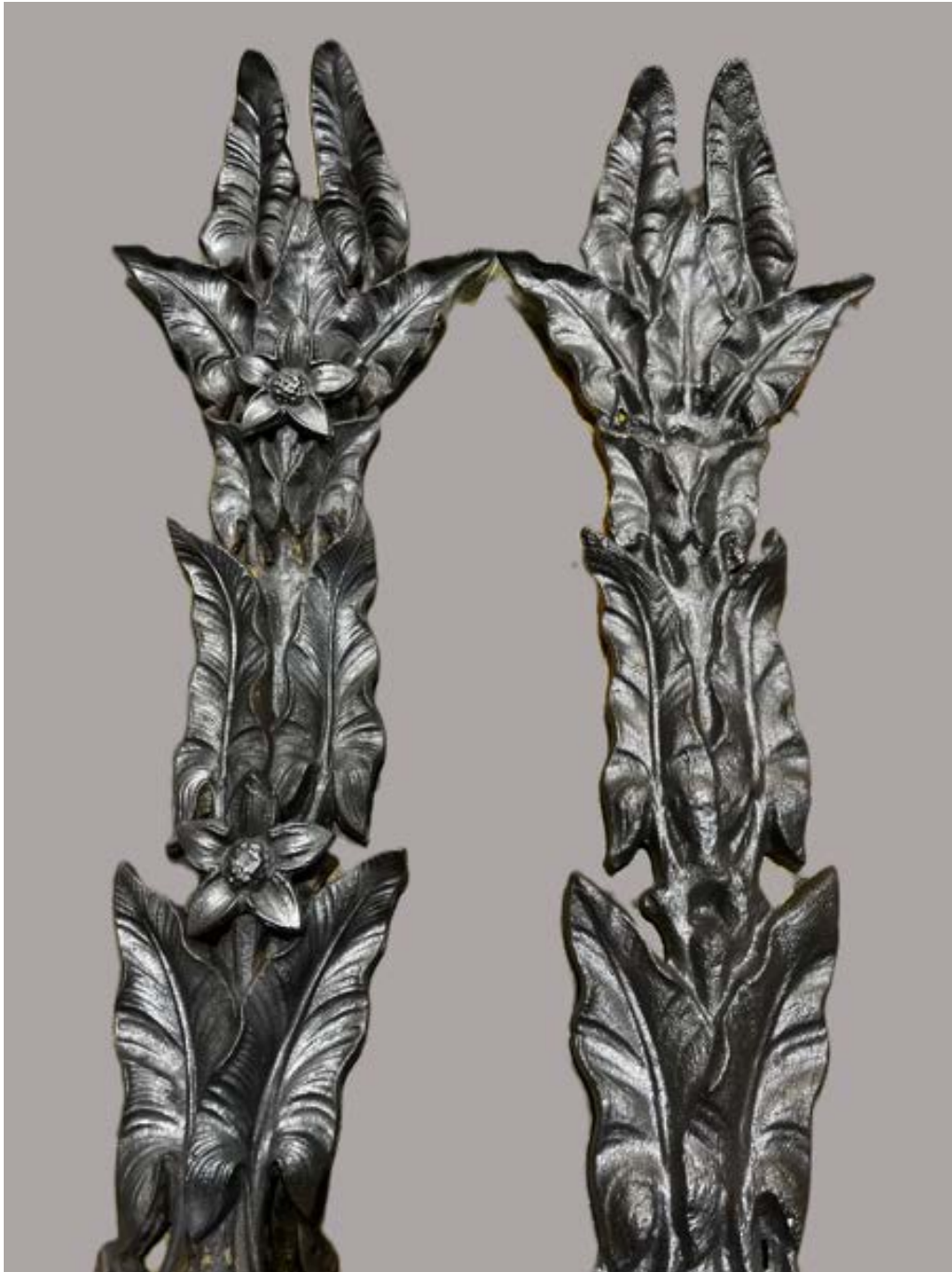
Figure 128 Photo showing the difference between the original casting and the new supplied casting. Quite a contrast in the lack of detail.
