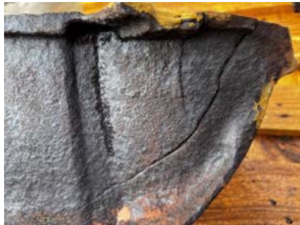
Figure 77 Photo showing the back of the left-hand side crack in the bowl
