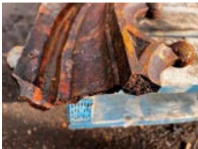
Figure 86a Photos showing the four broken sections of the face panels, each one proposes different challenges as to the repair method
