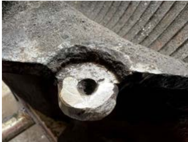
Figure 83 Photo showing a repaired bottom locating lug, this is to be threaded
