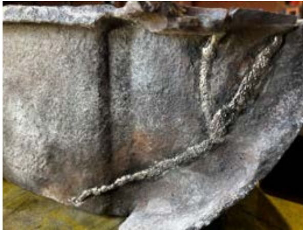
Figure 80 Photo showing repaired crack and peened weld on the bowl
