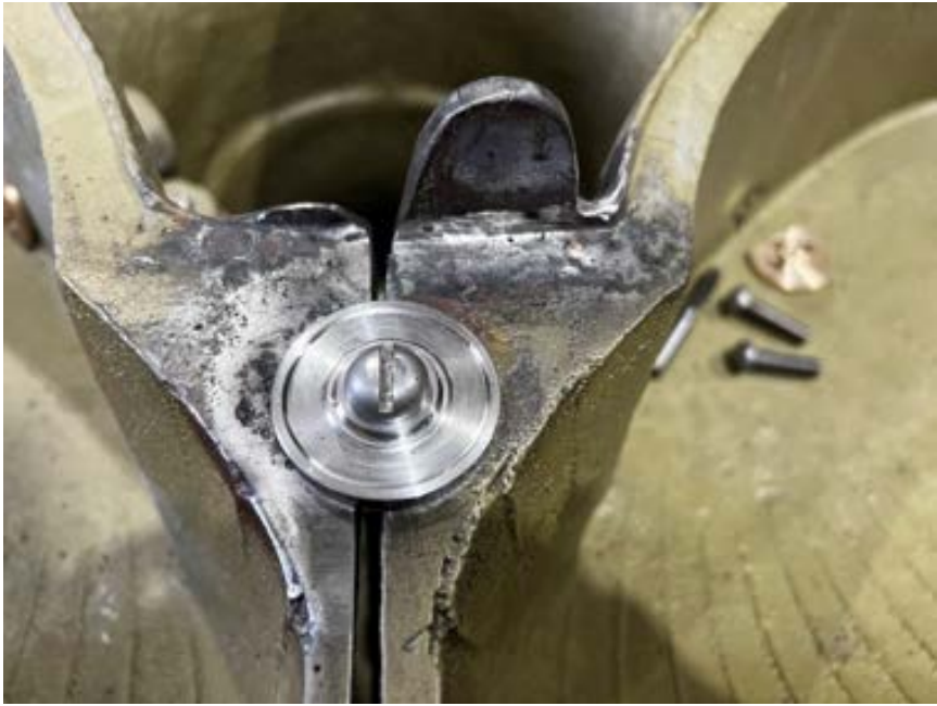
Figure 86 Photo showing the lugs and washers assembled
