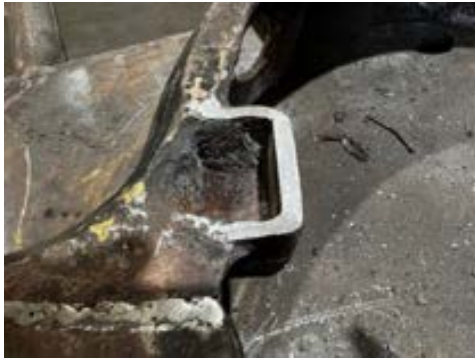
Figure 83 a & b showing repaired locating pockets for the fountain body
