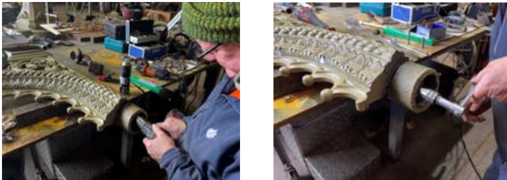
Figure 103a & b Photo showing Chris drilling and threading the retaining screw for the plug
