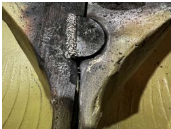
Figure 84 Photo showing a repaired top locating lug, this is yet to be drilled upon initial assembly
