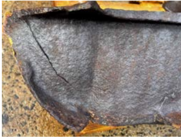
Figure 76 Photo showing the back of the right-hand side crack in the bowl
