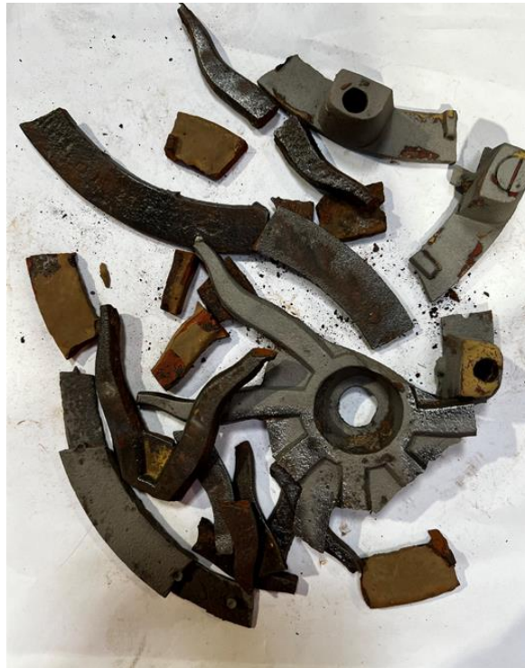
Figure 20 Showing the remains of the Radiating Sun Casting as it was delivered to Glasgow Engineering some sections were completely missing
