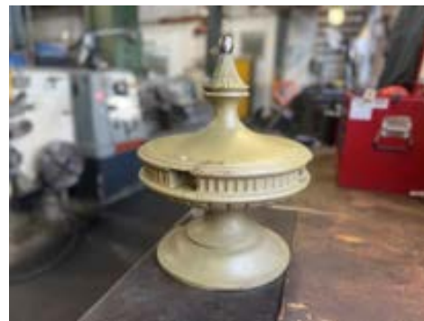
Figure 97 Photo showing new ball on top of the cup holder. The cup holder will require four new arms to be cast and four new location tabs to be attached.
