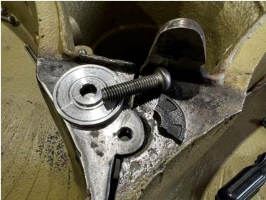
Figure 85 Photo showing completed locating lugs and 316 ss washer made to the same profile as the cast iron washer
