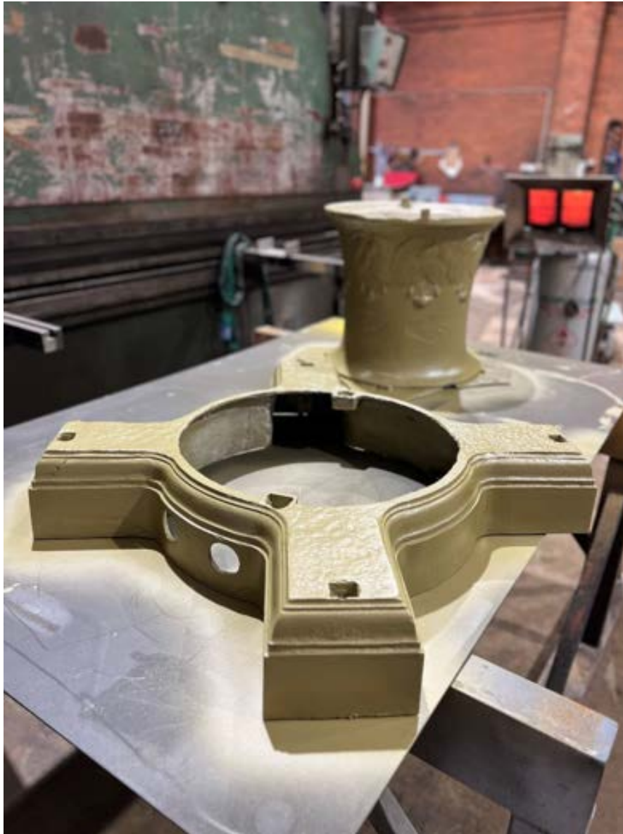
Figure 94 Photo showing repaired base, this will require further work in rectifying the corrosion on the top with an automotive body filler to stop water pooling in the pitting
