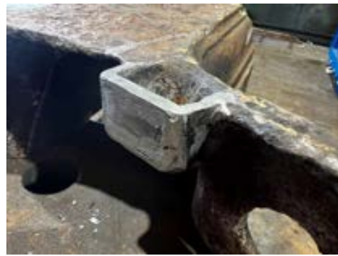
Figure 83 a & b showing repaired locating pockets for the fountain body
