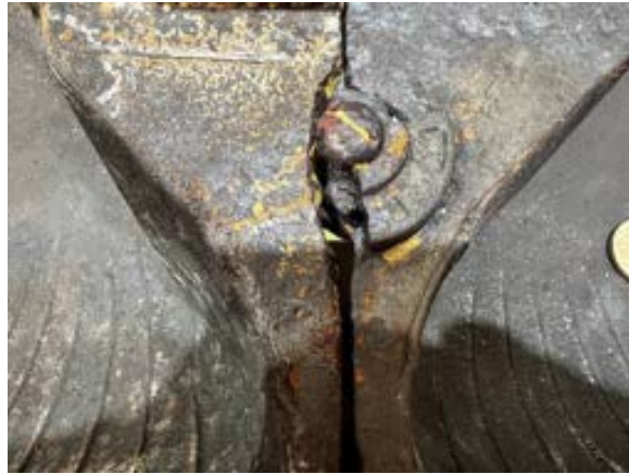
Figure 82 Photo showing one of the remaining screws and cast-iron washer that locates the four bowls. You can see from the photo that the top lug and washer is broken
