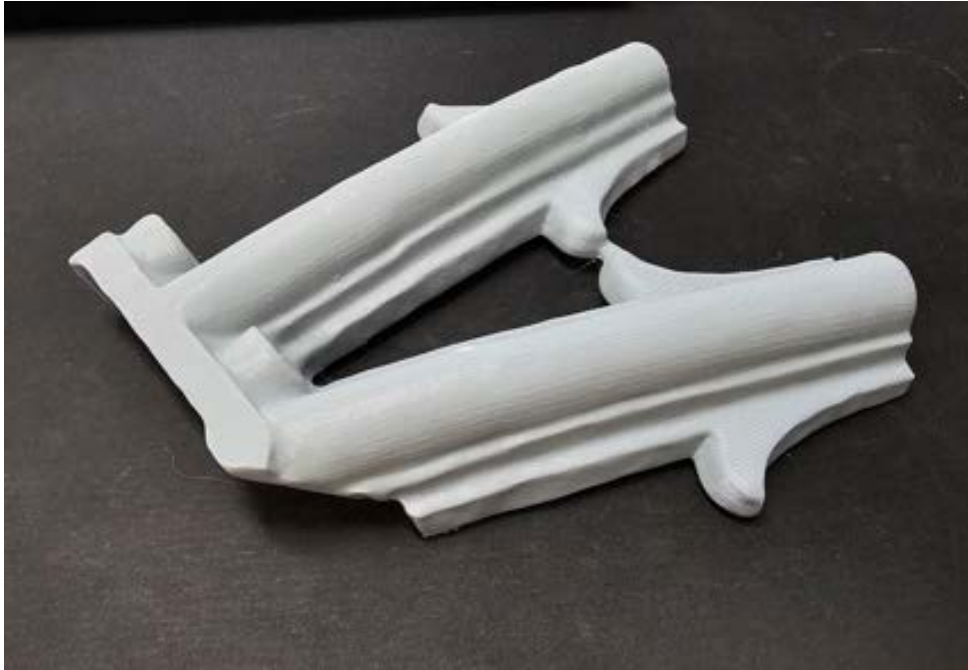
Figure 120 Photo showing 3D printed pattern
