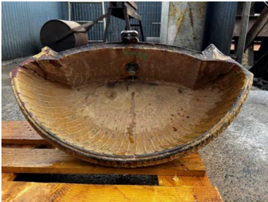
Figure 75 Photo showing the cracked bowl
