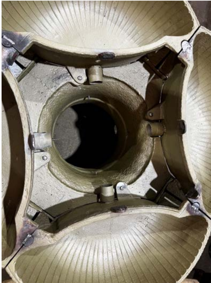
Figure 87 Photo showing the bowls assembled on to the base. Of the four main retaining lugs holding the bowls to the base only one was intact. You can see the interlocking tabs at the side of the bowls that hold them together, only two of the lower ones were intact, all the others had been broken off.
