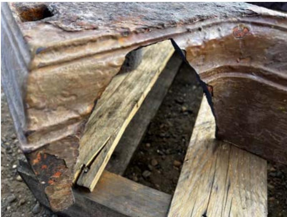
Figure 53 Photo showing historic broken section from the side of the base plate, this was an old, cracked section that broke free trying to remove the base
