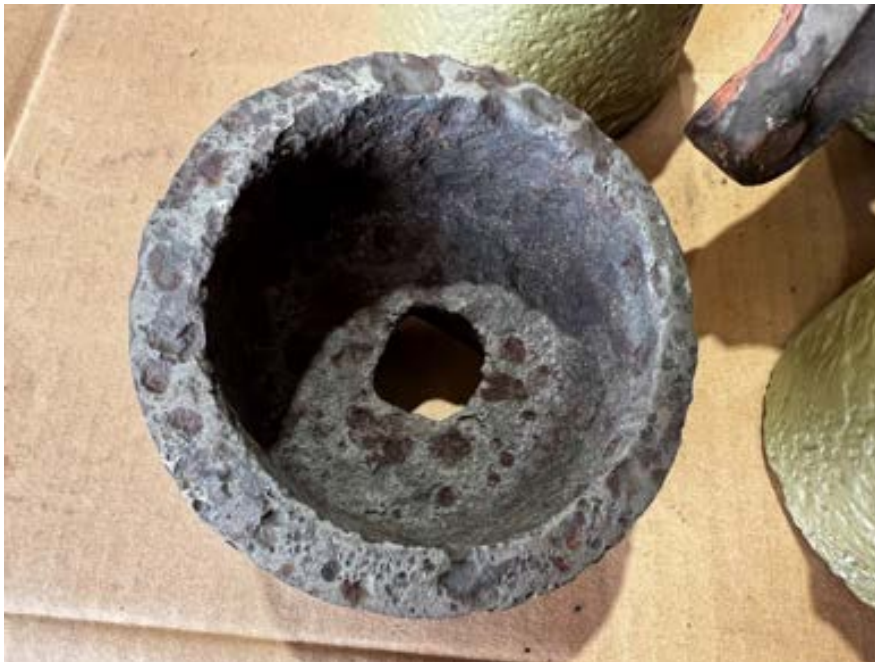
Figure 49 Show the cusped arch face panel plug with the square peg hole corroded through
