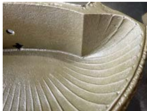
Photo 80a Photos showing both left hand and right-hand crack repair completed and dressed
