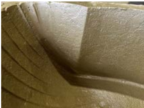
Photo 80a Photos showing both left hand and right-hand crack repair completed and dressed
