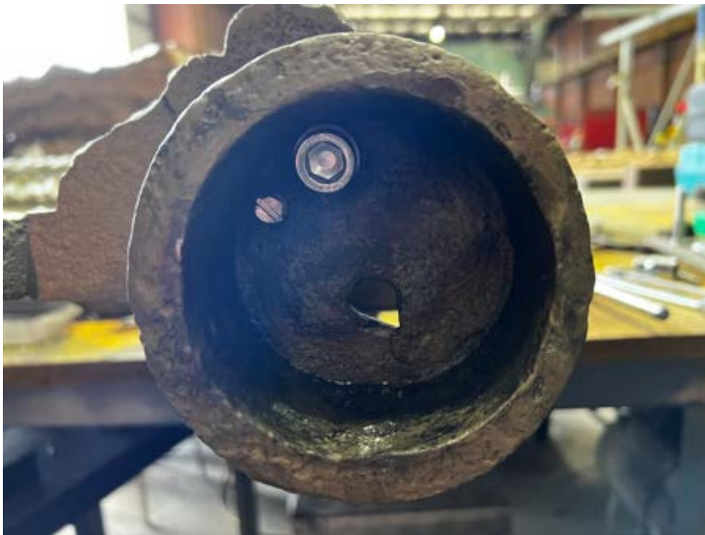
Figure 104 Photo showing the M12 retaining screw and the M10 locking screw
