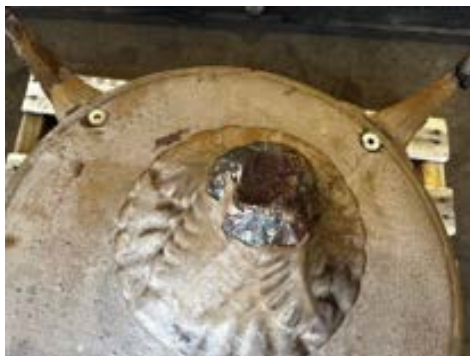
Figure 97 Photo showing new ball on top of the cup holder. The cup holder will require four new arms to be cast and four new location tabs to be attached.
