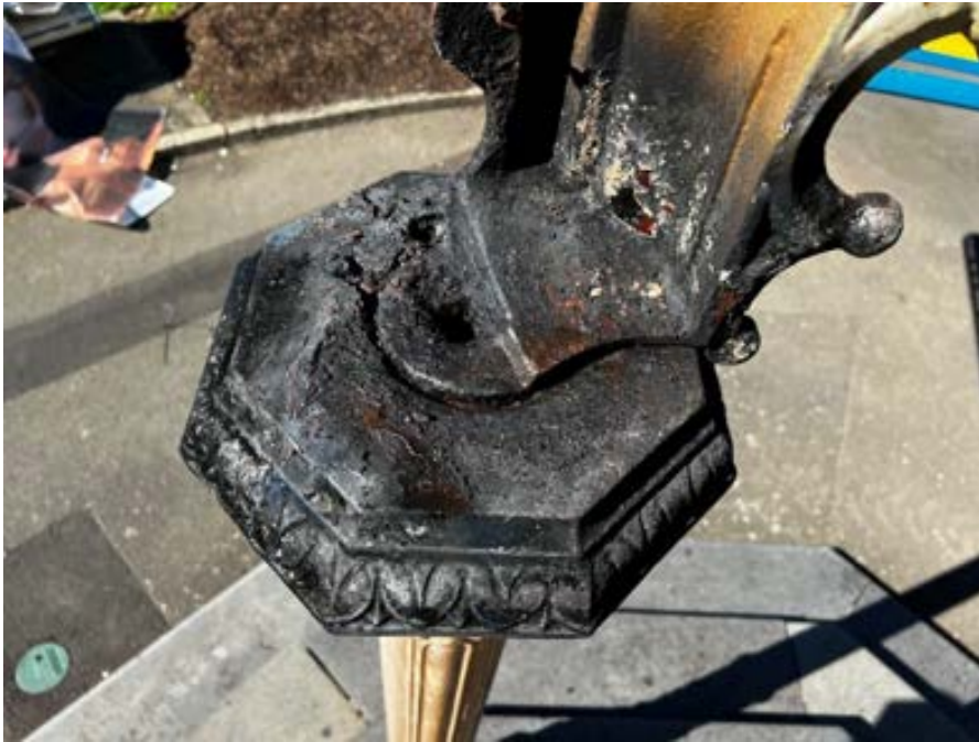
Figure 38 Shows the amount of heat required to remove the plug from the socket
