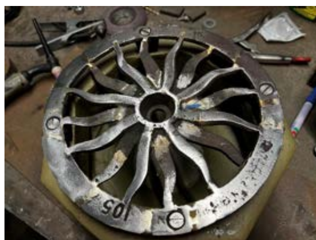
Figure 111 Photo showing repaired sun casting
