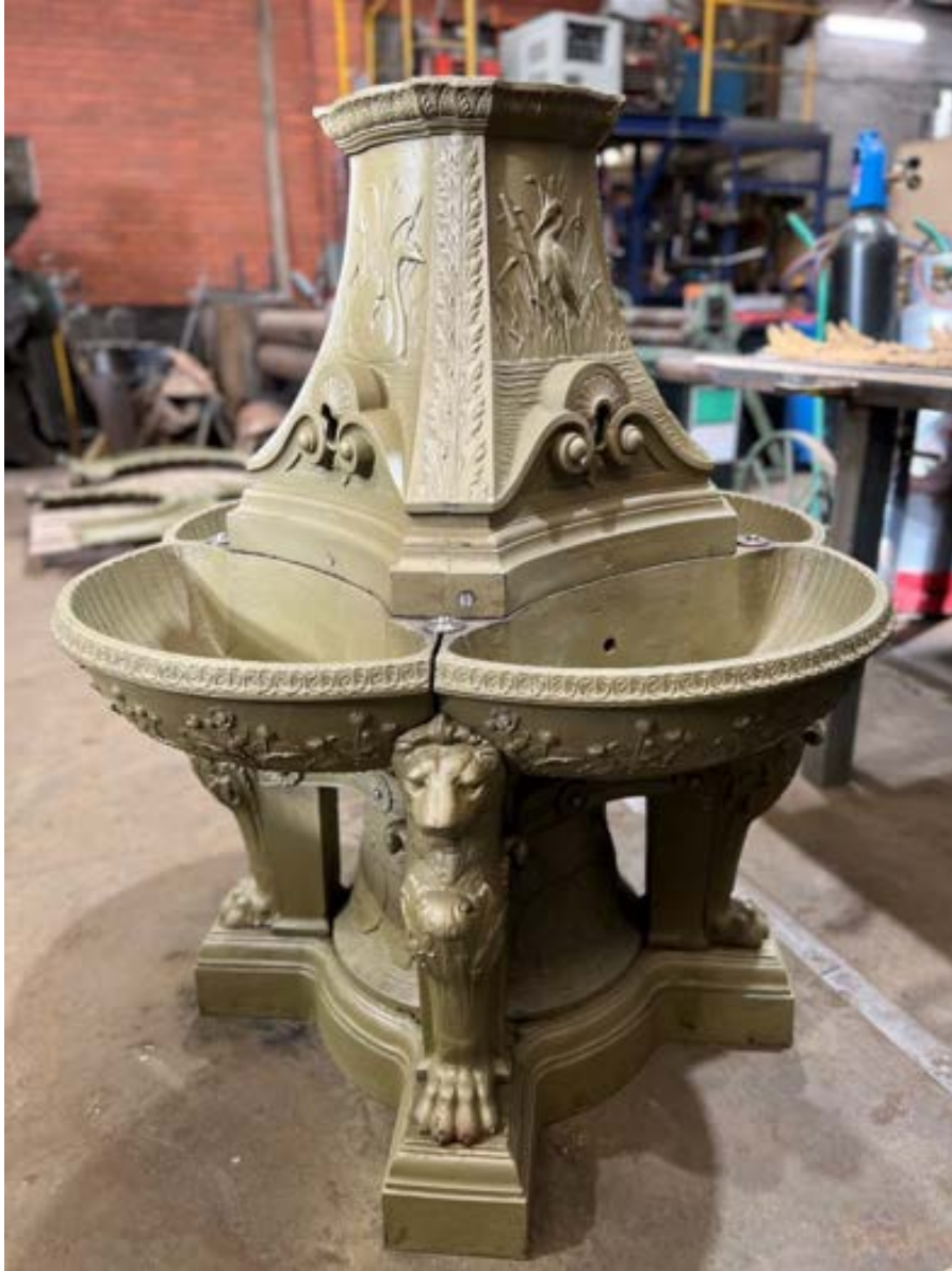
Figure 98 Photo showing the drinking font partially assembled to check fitment
