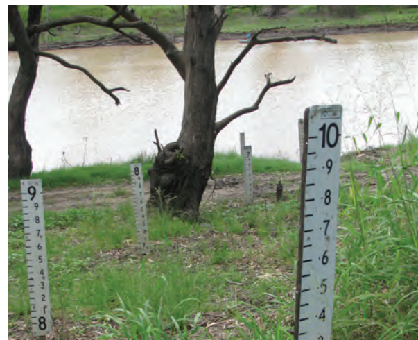
Flood gauges on the Balonne River at St George, early 2012. Source: QldRA
