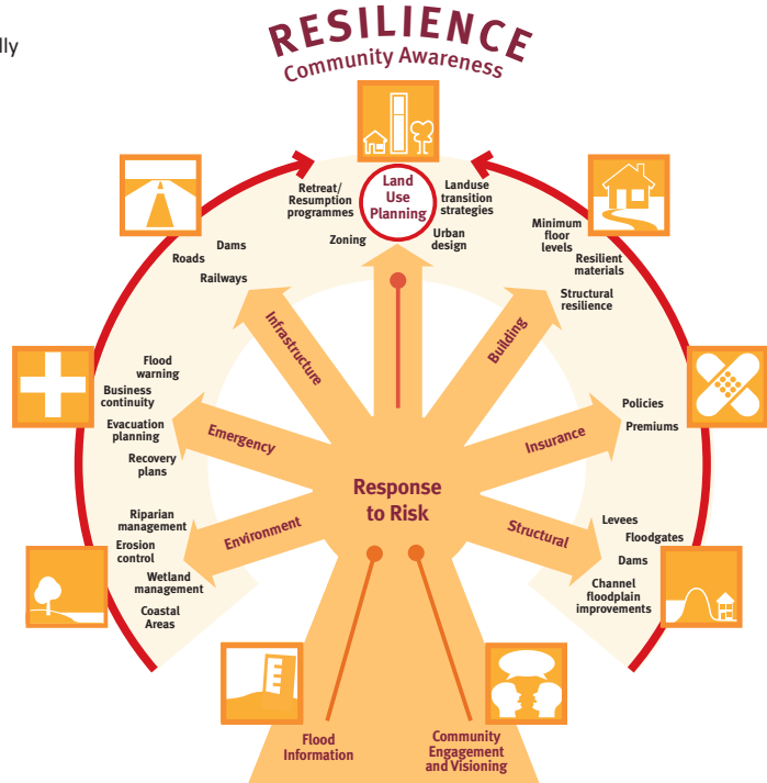
Figure 1: The floodplain management process provides a comprehensive suite of measures that contribute to building resilience in the floodplain.
