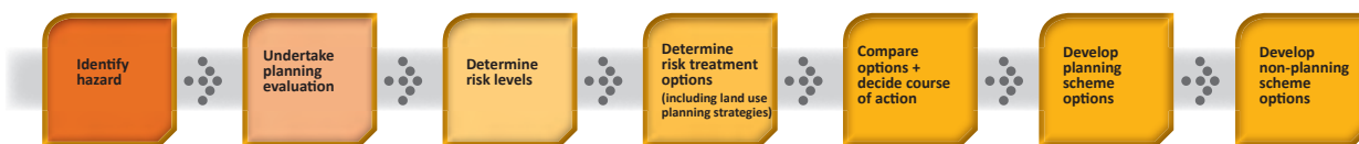
Figure 22 – The process workflow for undertaking a planning evaluation using the hazards identified through the flood investigation previously selected and prepared.
