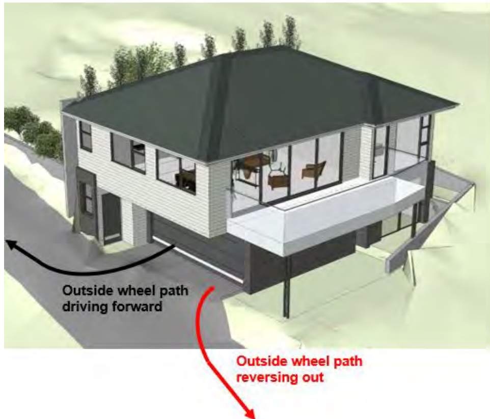
Figure 25 – 3D view of ROW access to proposed 18 Wyett Street unit
