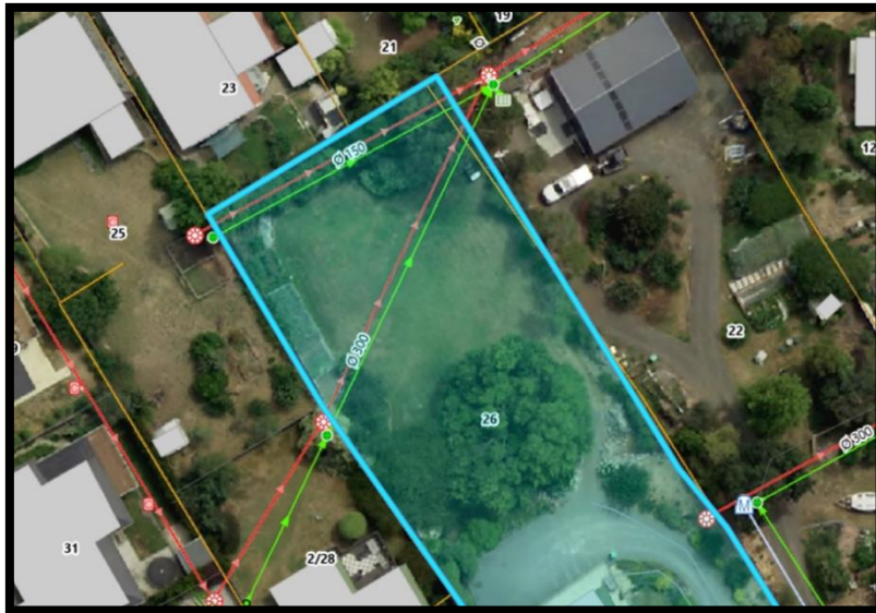
Figure 4 - Sewer and Stormwater Drainage Infrastructure
