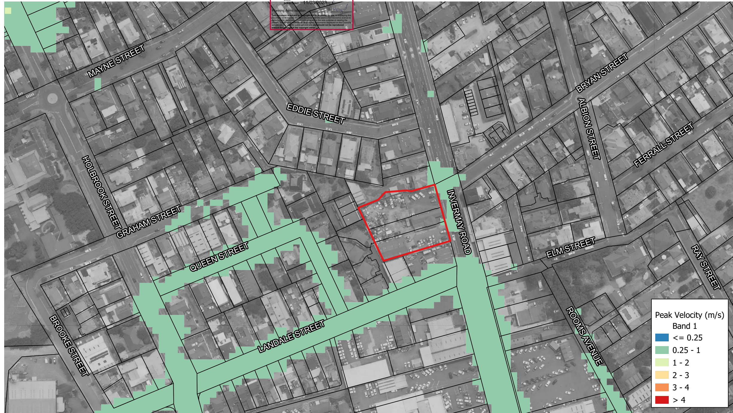
Figure A12: Levee Breach Scenario - 1% AEP - Peak Flood Velocity
