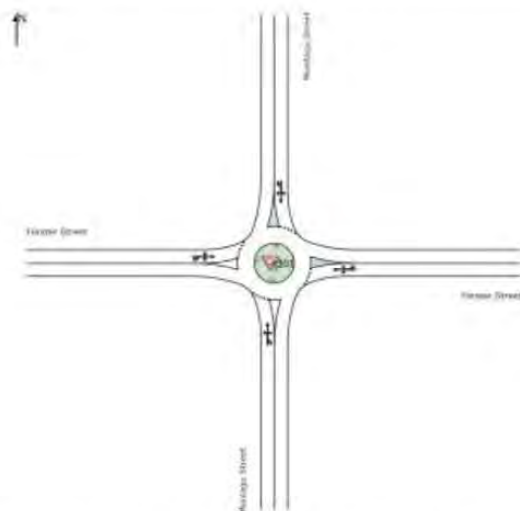
Figure 6: Geometric layout – Montagu Street/ Forster Street roundabout
