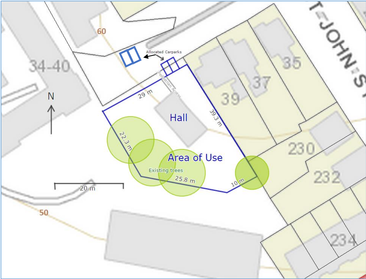
Figure 2 – Detailed plan of the site showing the dimensions of the area; existing building; existing vegetation; contour lines; title boundaries and street access.
