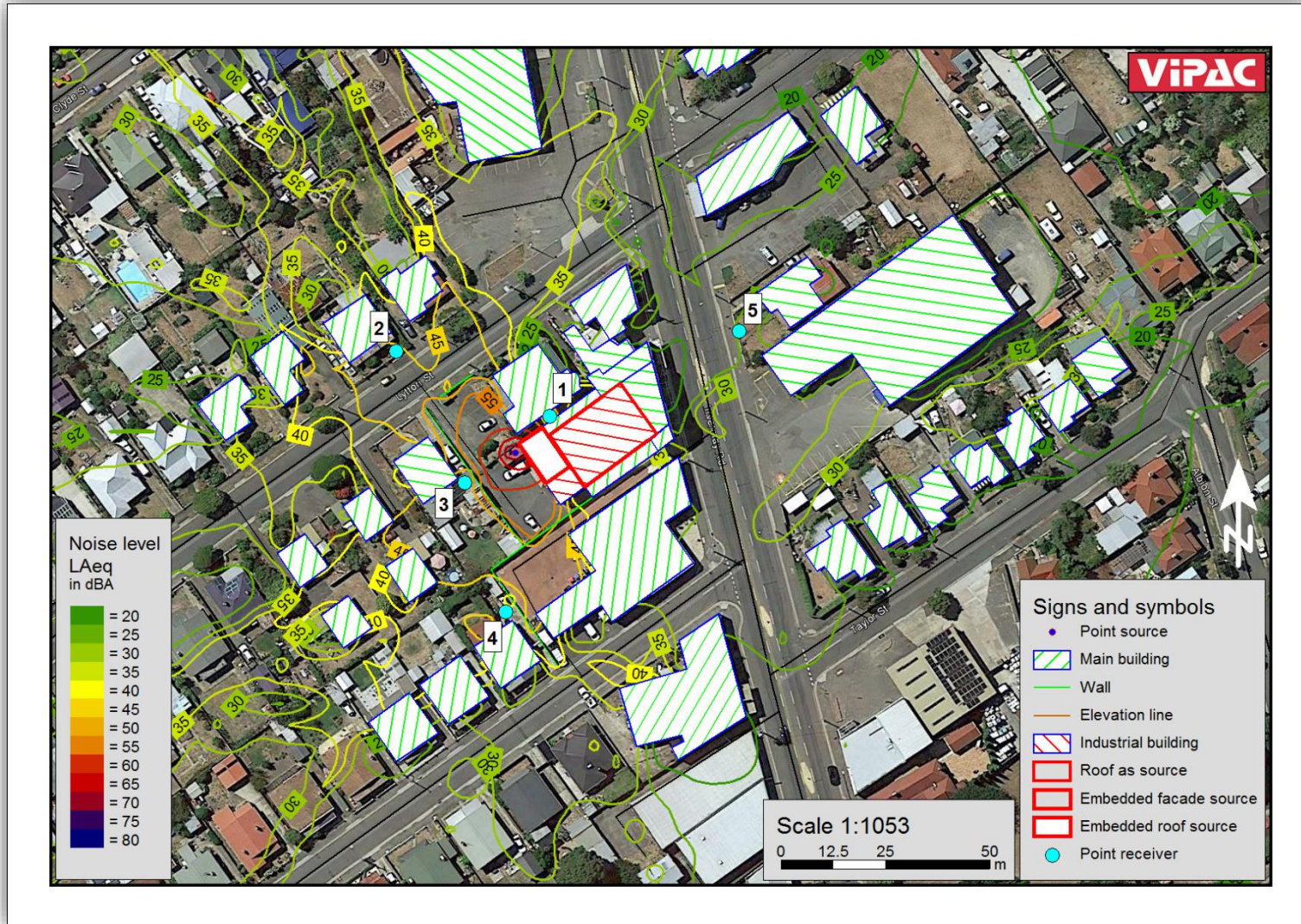
Figure 9 – Predicted noise emission contours, cinema showings, mechanical plant in carpark – 1.5 m above ground height.
