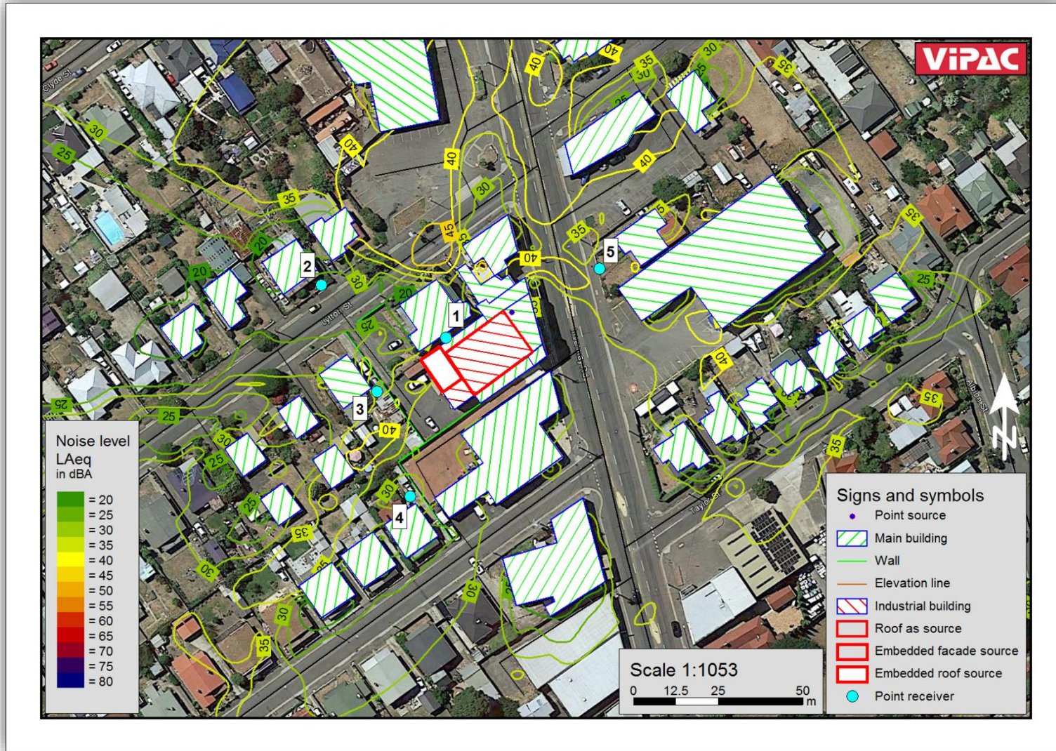
Figure 7 – Predicted noise emission contours, cinema showings, mechanical plant on roof – 1.5 m above ground height.
