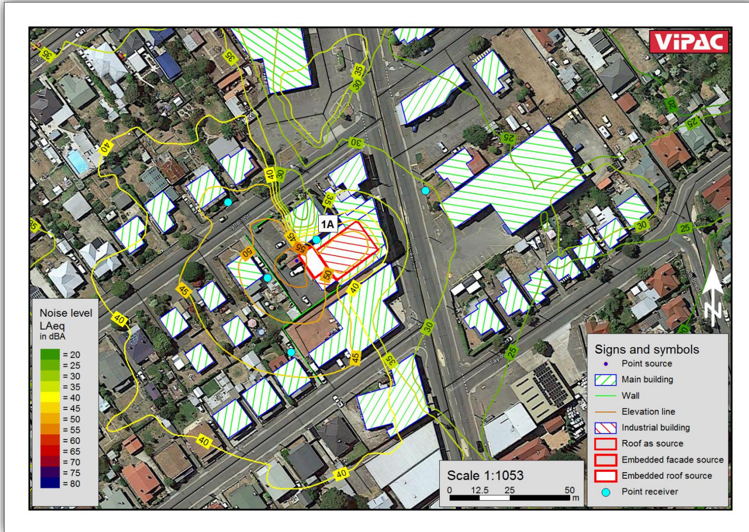
Figure 10 – Predicted noise emission contours, cinema showings, mechanical plant in carpark – 5.5 m above ground height.
