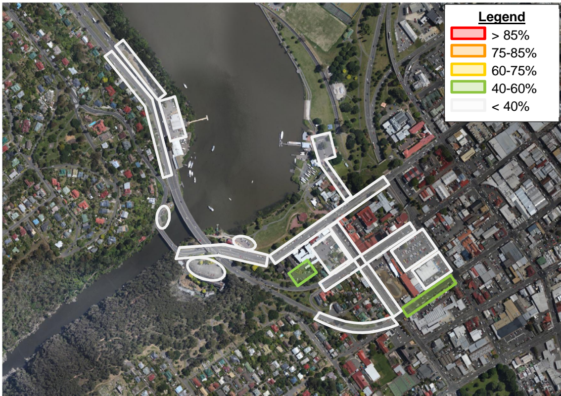
Parking Occupancy (%) at 7:00 am Thursday
