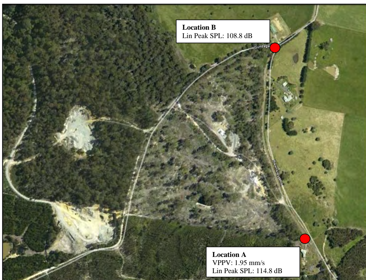
Figure 4 – Aerial view of Gundagai Quarry and surrounds with ground vibration and air blast overpressure data presented at the measurement locations.
