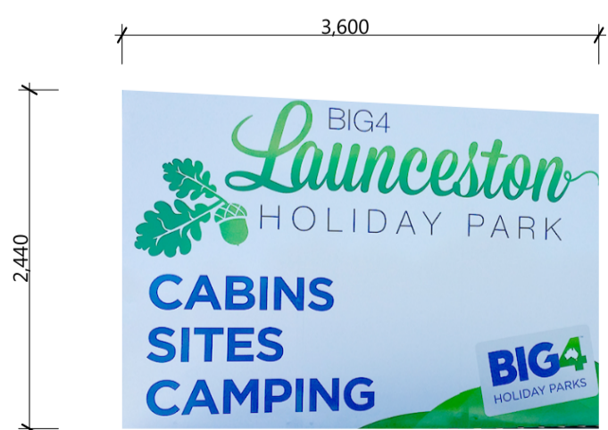
SIGN B EXISTING SIGN MOUNTED TO NEW PYLON WITH GROUND MOUNTED FLOOD LIGHTING MAX 6m HIGH
